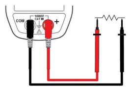
An audible signal is emitted if there is continuity (resistance value is below the maximum threshold - see § 3.4.1) and the measured value is displayed on the screen.
