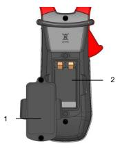
Figure 6 : The Battery Compartment
