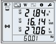
Real-time updates are displayed for voltage (V), current (I) active power (P), reactive power (Q), apparent power (S), frequency (Hz), power factor (PF) and phase shift (φ).
