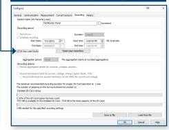
Configure the PEL to measure and record over a user selectable recording period. Select demand intervals and view available memory for data storage on the Recording tab.
