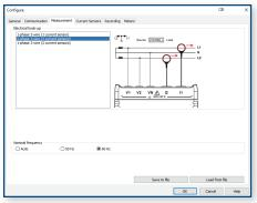
The Measurement tab specifies the electrical distribution system, voltage ratios, nominal frequency and current probe options and ratios. NEC 220.87 load study checkbox initiates the recordings to accurately meet requirements.
