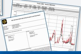
Reports can be viewed on a PC and printed. They contain test results in tables and graphics, along with operator and test site details. Operator comments are also included.
