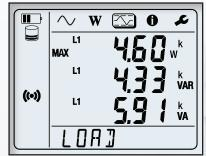
Max aggregated values of measurements and energy.
