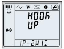
Hook up, Wi-Fi, aggregation period, can be configured from the front panel of the PEL 52. Current ratios and number of turns need to be configured via the PEL Transer software based on the current sensor type.
