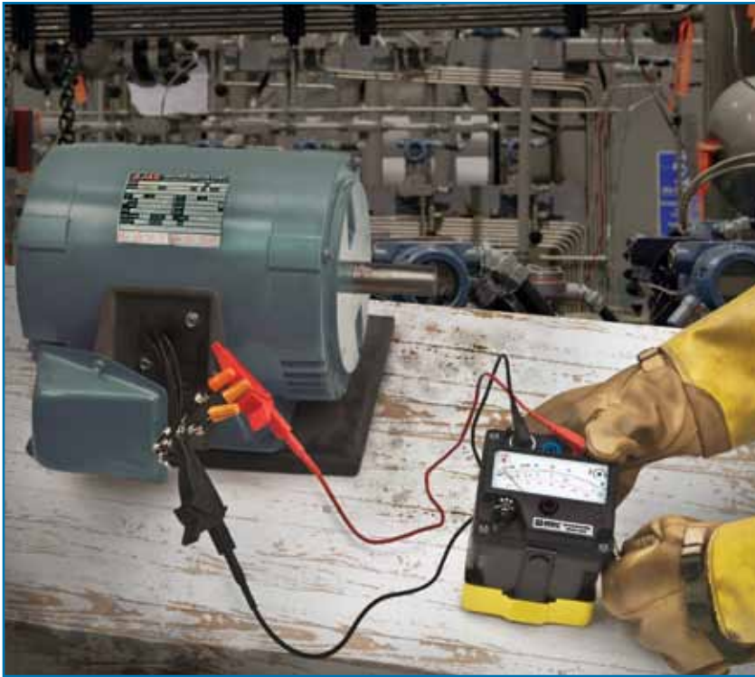
Model 6503 performing a hand-cranked 1000V test on a generator.
