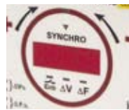
LED display of 3 measurements: phase, frequency and voltage
